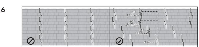
Alternate the joints between rows. For a nicer look, we suggest alternating the cutting distance of the first section of every row from 0"(0cm) - 15"(38,1cm) - 30"(76,2cm) - 28"(71,1cm).
