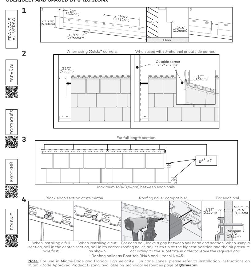
Install sections and space equally. Refer to temperature marks that show the outside temperature the closest to that during installation.
