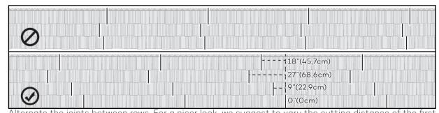
Alternate the joints between rows. For a nicer look, we suggest to vary the cutting distance of the first section of every row from 0"(0cm) - 9"(22,9cm) - 18"(45,7cm).- 27"(68,6cm).
