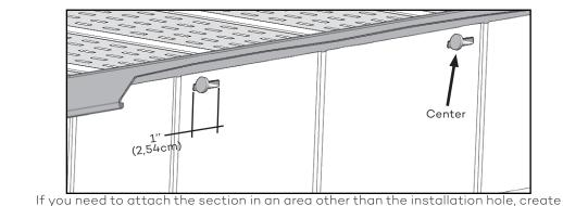
a 1"(2,54 cm) long slot to allow nailling. Always nail in the middle of the slot.
